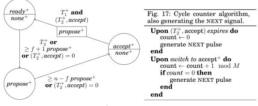
Fig. 16. The quick cycle of the FATAL<sup>+</sup> protocol.
